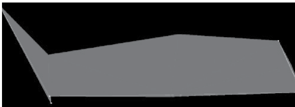
Figure 8. Enlarged view of poor quality elements.
