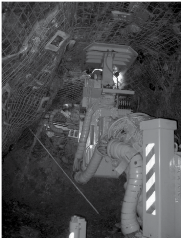
Figure 2. Fletcher model N3114-AD/E Roof Bolter in operation.
