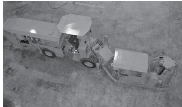
Figure 3. Basket swing can be used to keep the basket parallel to the slope when the boom is swung.
